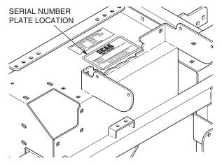
Figure 1-1. Mower Serial Number Plate Location
